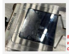
Mould residuum when moulding competitor material
